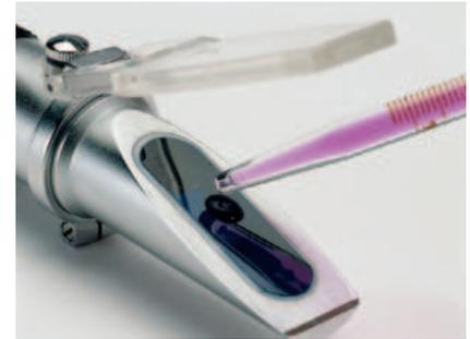
**REFRACTÓMETROS PARA LA SALINIDAD ‰ Y DENSIDAD “C-1”**
