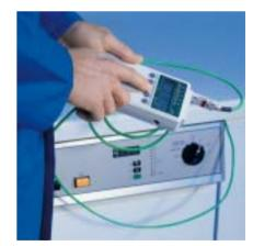
Access point for measuring temperature holding times
